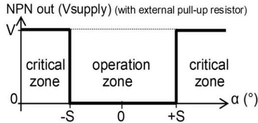
The default  $0^\circ$  position is when the sensor is mounted horizontally (label upwards) and no acceleration is applied.
